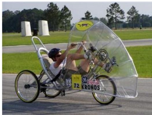
*Figure 9. University of Alabama's human powered vehicle with a partial fairing.*
