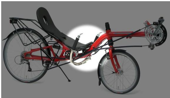
***Figure 6: Under Seat Steering***
