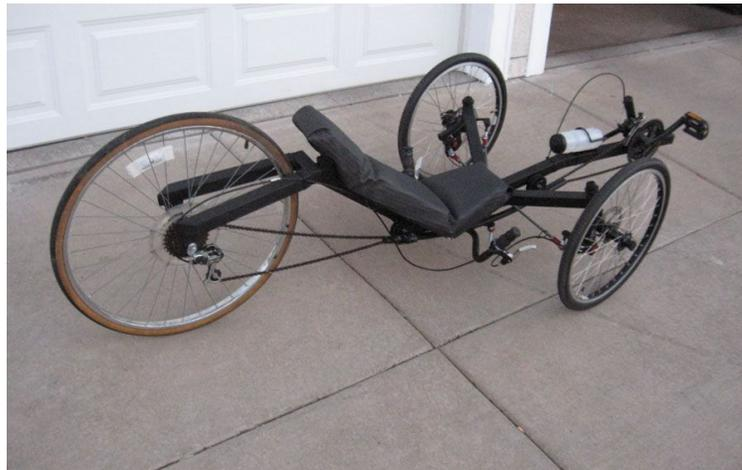
***Figure 4: Recumbent trike with Square Tube Frame***
